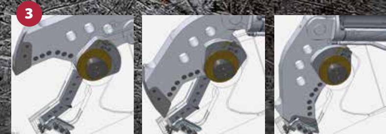
Shear Arm Guiding System (SGS)
